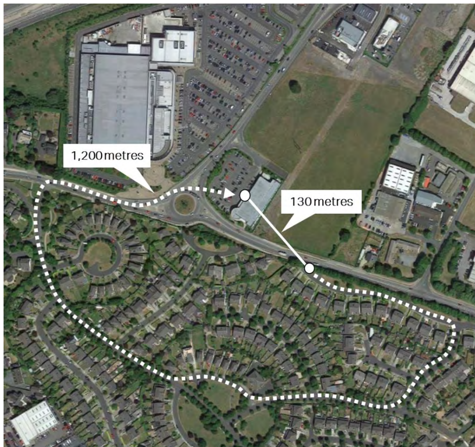
Figure 4.28: Example of Indirect Travel due to Cul-De-Sac Design and Boundary Walls
